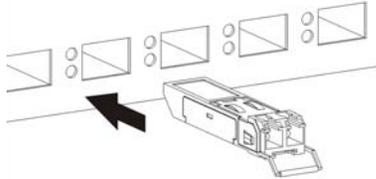
**Figure 12** Connecting the Fiber Optic Cables
