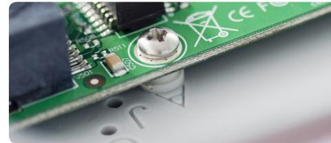
3 Install selected board using spacers and screws.
