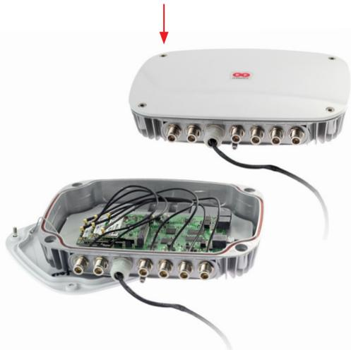
5 Close the enclosure and tighten the screws.
