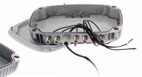
2 Remove red silicone caps and install desired amount of pigtailed connectors. Use only sealed pigtailed connectors (with O-ring).
